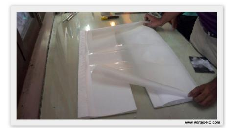
you move towards the leading edge, press the lamination roll firmly onto the wing.
