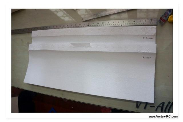
C. Lightly sand the wings before laminating to get a better adhesion. Very gently and uniformly sand using the supplied sandpaper keeping the wing panel on its bed. . Idea is to just remove the thin outer brittle layer of foam . After sanding, clean up the wing with a cloth.
