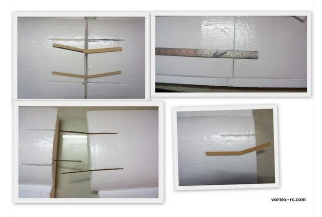
carefully before gluing. After glueing, inspect the joint carefully, and apply some packing tape to the joint to ensure it doesn't move while the epoxy cures. Be sure to keep one wing panel propped up.
