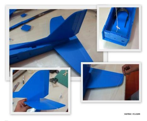
Install the skids as shown below. Flow CA glue through the joints to ensure these are properly glued in.
