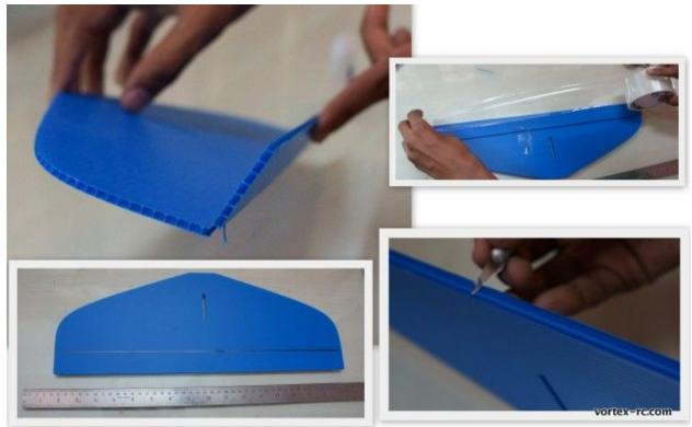
Likewise prepare the rudder by scoring a line 3.5 cm from the aft line. Follow the same technique as with the elevator to create the Rudder hinge.
