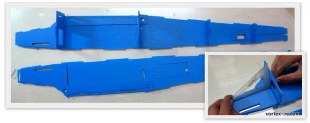
Next, Take the Wing mount plate, and align it correctly. Test fit it into the notches within the fuse, and the Former B and C. Take time to fit it as accurately as possible. The Wing mount plate fits only from one side. So be sure to align properly. Add CA to secure the plate in position
