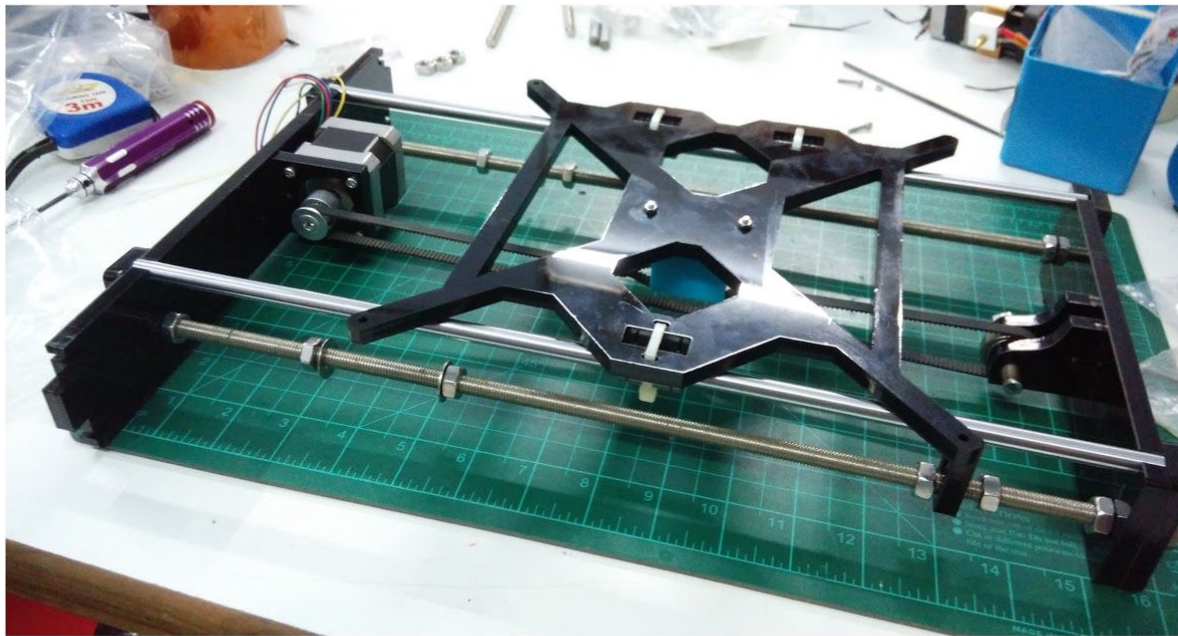
Completed Y-Axis assembly
