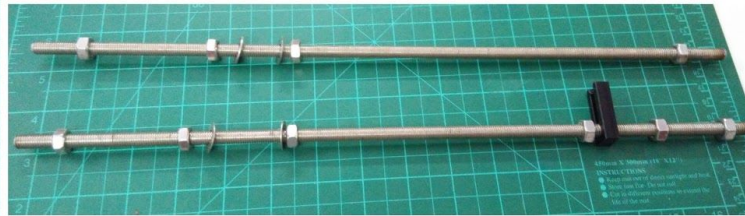
Threaded Rods with M8 nuts, washers and limit switch holder in place
