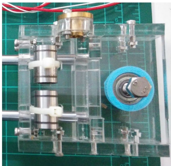
Linear Rods go through Part A and B on both the X-Axis motor mount and Idler
